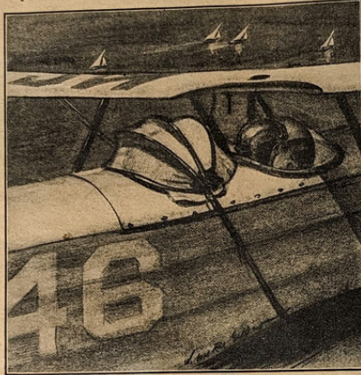
Picture by William MacRae Gillies How blind flying is taught. The student pilot sits in the hooded rear cockpit.
