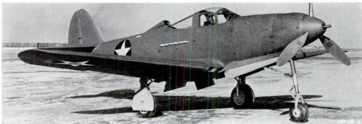
Now going into Army service are Lockheed P-38, above, and Bell P-39, below. Both are powered with Allison engines. Each is armed with a 37 mm. cannon in addition to numbers of .30 and .50 caliber machine guns.
