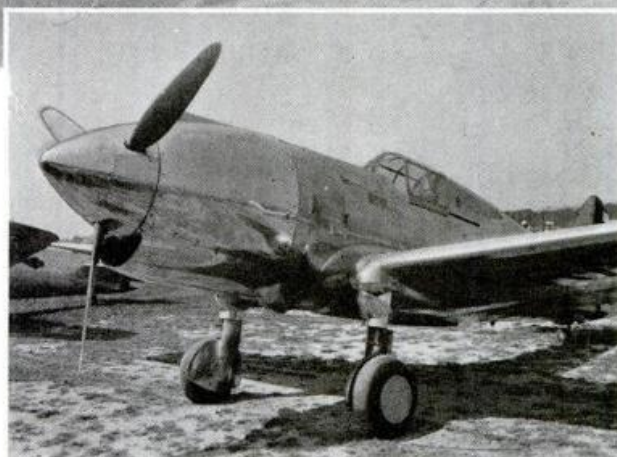
Standard "conventional" Army pursuit is the Curtiss P-40 above. It is an Allison-powered successor to the P-36A which it replaces. XP-42 (right) was experimental P-40 with an extended-shaft radial.
