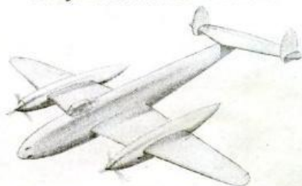
Conventional fuselage with twin tail unit.
