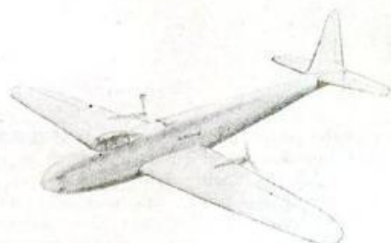
Fuselage engines side by side, pusher props.
