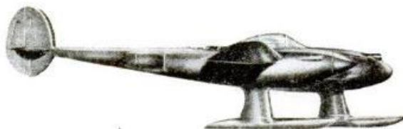
One P-38 ski plane with full-retracting skis was built.
