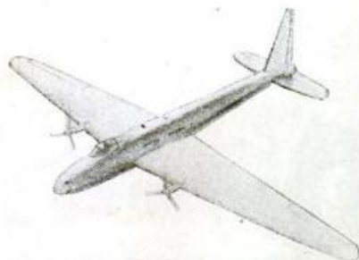
Engines in fuselage, geared to props in wing.
