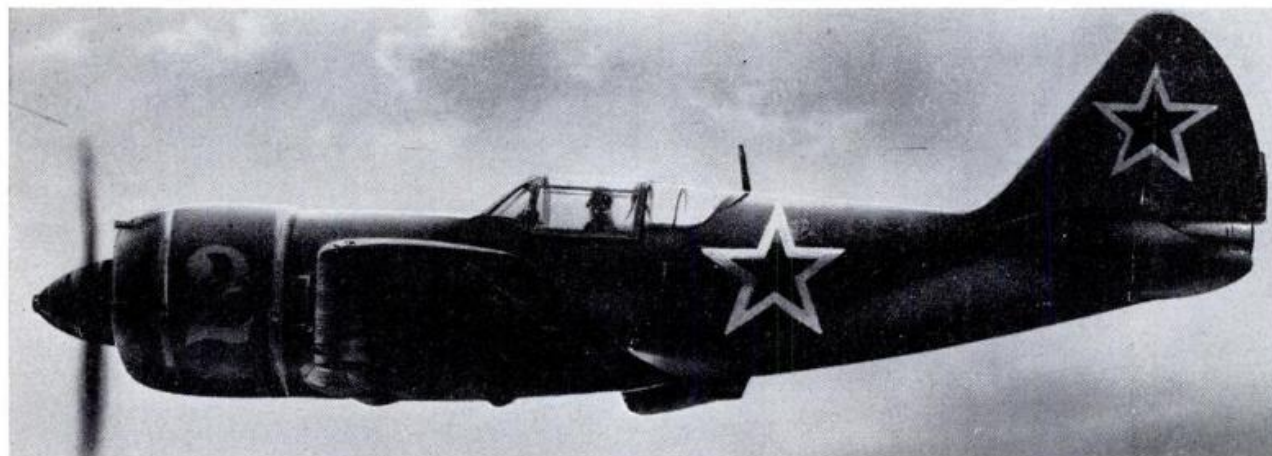
EXPERIMENTAL version of Lavochkin La-9 has liquid rocket unit in rear fuselage with exhaust efflux orifice below modified rudder. Another La-9 has been fitted with impulse duct motors under each wing. It is unlikely that any of these machines entered squadron service.
