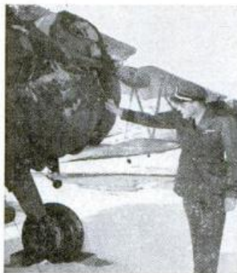
Engine covers are "must." Plexiglas, propellers also need covers.
