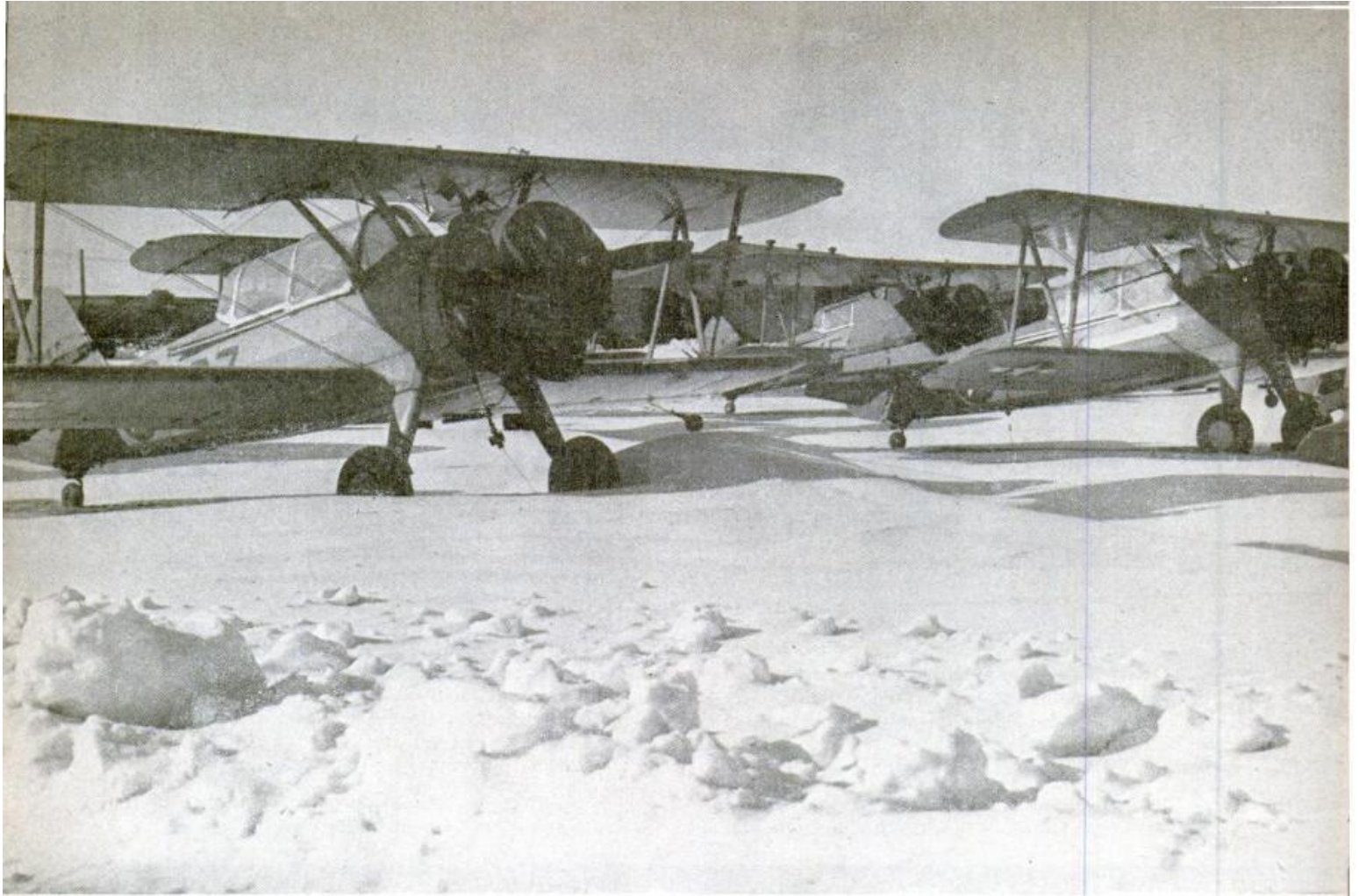
Only engine hoods protect Navy's fabric-covered Boeing N2S trainers, yet they are ready to fly when the snow is cleared away.
